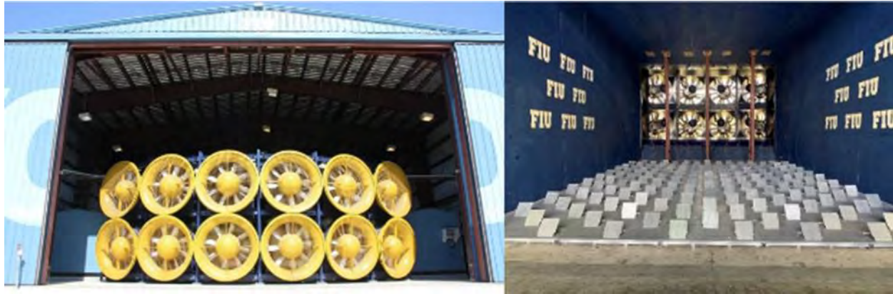
Figure 1: FIU NHERI Wall of Wind experimental facility showing (a) rear end consisting of 12 fans positioned in an arch shaped, 2 rows by 12 columns and (b) front end consisting of the flow management box shooting the ABL wind flow jet.
