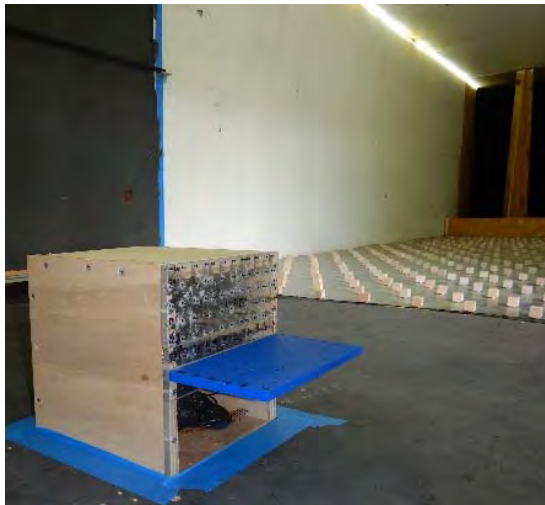
Fig. 3: Model-3 in the wind tunnel and a plan view of the model showing 0-360-degree wind direction
