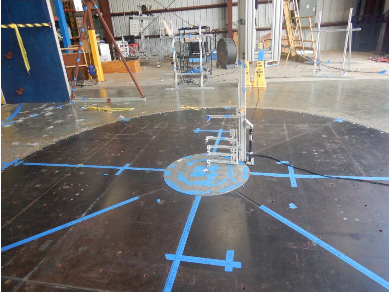
Figure 5: Location of the cobra probe to measure wind velocity
