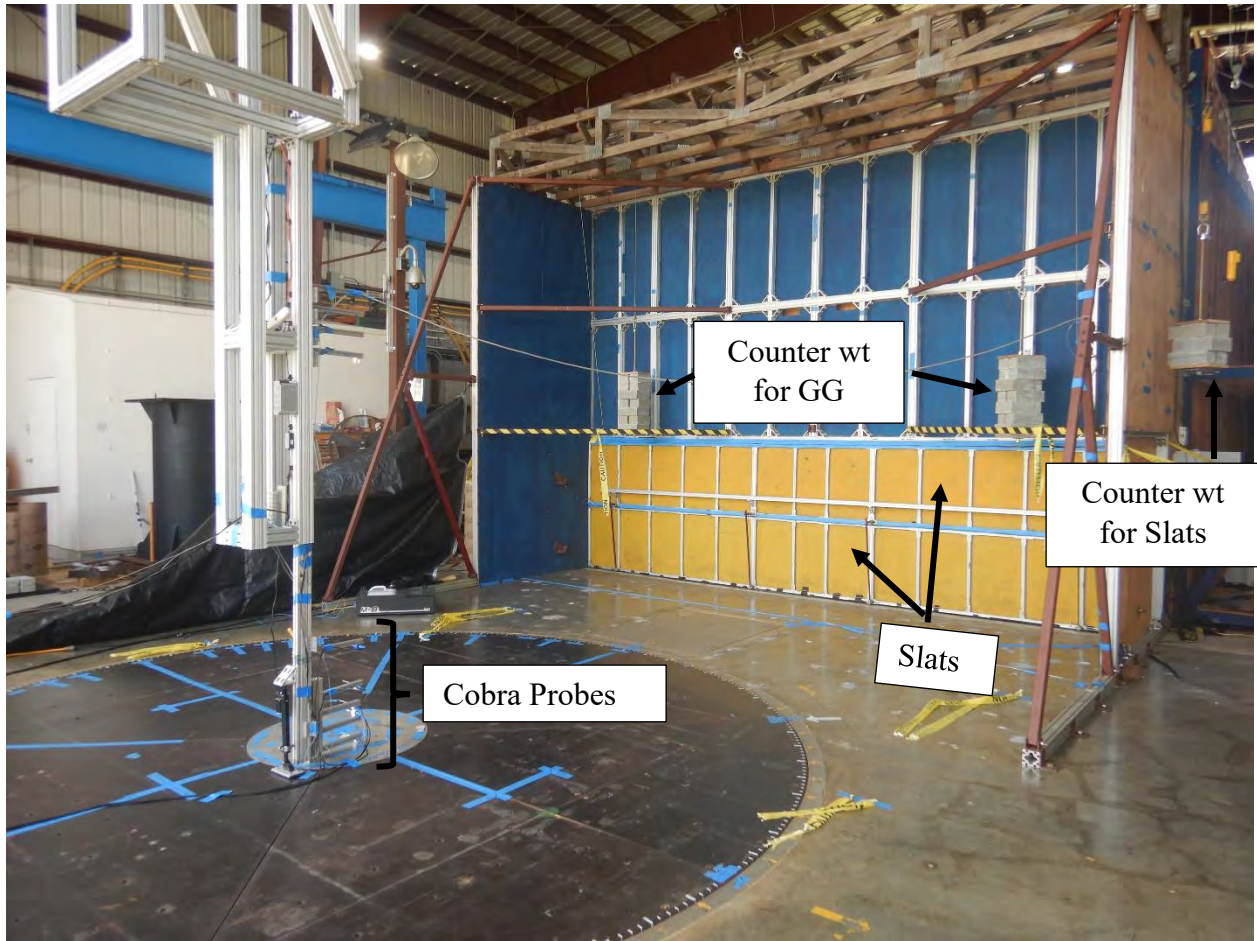
Figure 2: The WOW downburst simulator with the Cobra Probe at the Turntable Center
