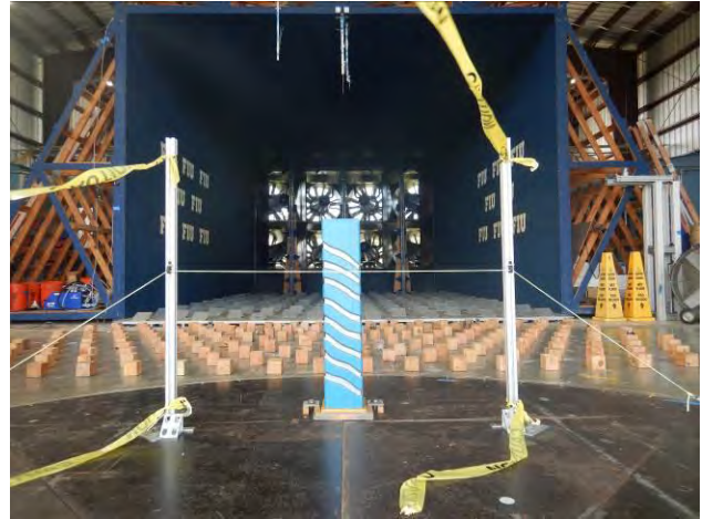
Wall of Wind building model test set-up.
