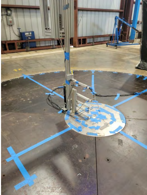
Figure c: Cobra probe location at the turn table center
