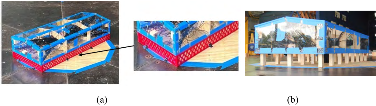
Figure 6. Isolated MH model with (a) partially-enclosed crawl space and (b) open crawl space
