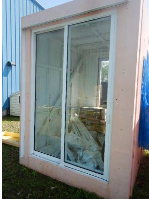
Figure 2. Large-scale building model with full-scale sliding glass door
